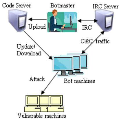
Fig. 1. A typical IRC-based botnet architecture
